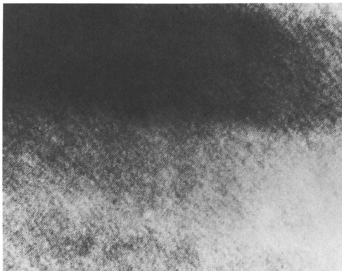
Figure 3. High resolution transmission electron microscope (111) lattice image of the same structure in Figure 2. The light and dark areas are the GaP and \text{GaAs}_{0.18}\text{P}_{0.82} layers which are horizontal. The light lines which are diagonal are the (111) lattice planes. The distance between the planes is \sim 3.16\text{\AA} .
